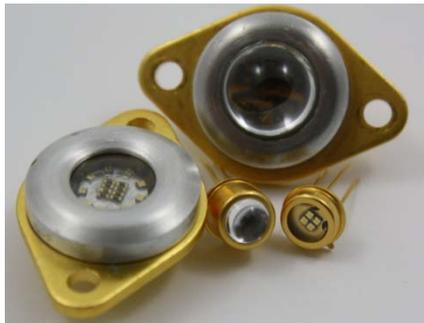
SETi's UVClean® LED array technology has been incorporated into the Psoria-Light's patent-pending emitter, which enables a compact handset to deliver very high power deep UV light in the range from 300nm to 320 nm; the optimum wavelength range for a variety of phototherapies. Psoria-Light systems are sold to dermatology healthcare providers for targeted UV phototherapy.
