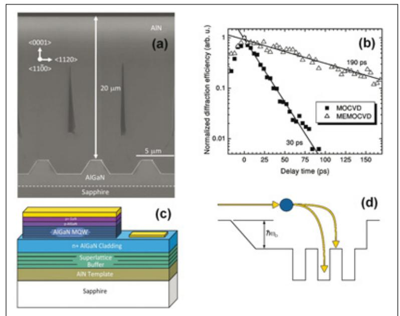
Figure 2 (a) SEM micrographs of a fully coalesced 20  $\mu\text{m}$  thick AlN sample grown by MELEO (b) Light-induced transient grating (LITG) decay in MOCVD and MEMOCVD-grown AlGaIn epilayers for the grating period of 7.7  $\mu\text{m}$ . Carrier lifetimes were estimated by fitting the decay transients with single exponents (lines) (c) Typical deep UV LED design (d) Schematic band diagram of DUV LED for capturing electrons in the light emitting region
